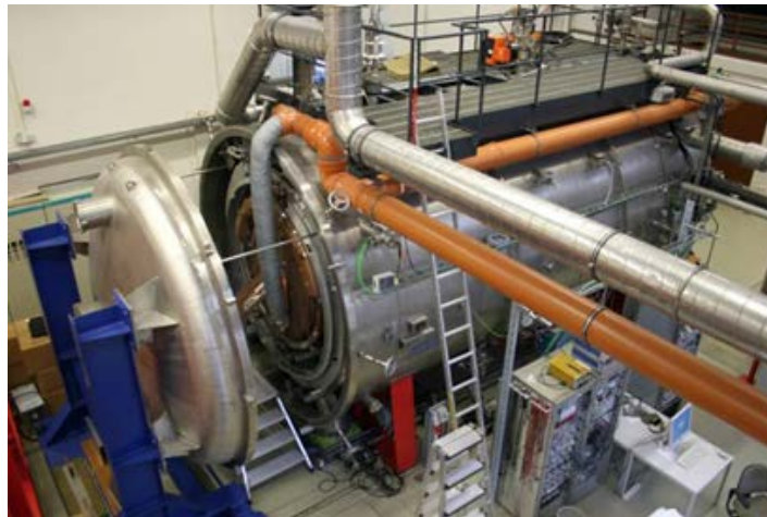
Figure 1 – STG-CT, high vacuum plume test facility
