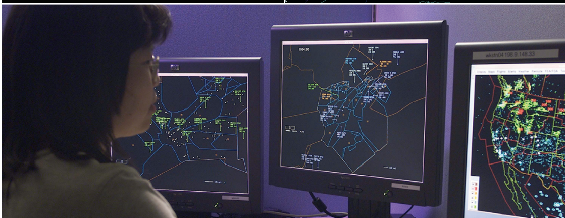
Images (Clockwise, left to right) Future Air Traffic Management Concepts Evaluation Tool (FACET) : A powerful computer simulation tool combines live air-traffic feeds and real-time weather data to display thousands of aircraft trajectories. Performance Data Analysis and Reporting System (PDARS) : Vividly displayed flight-track and flight-plan data help U.S. air traffic controllers monitor U.S. airspace and adapt to changing conditions. Traffic Separation Tools : New automation tools for aircraft flight decks and air traffic controllers will help more safely and efficiently adjust trajectories in a more crowded airspace.
