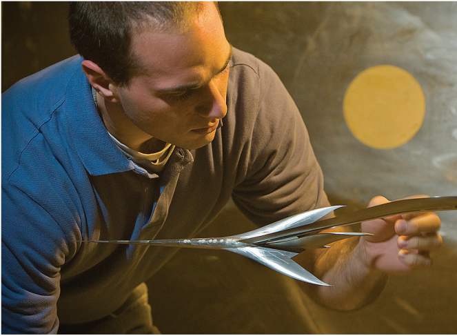
Test engineer Mark D 'Aprile checks a small model of a supersonic jet concept designed by Gulfstream Aerospace and tested in a NASA wind tunnel. Image credit: NASA Langley/Sean Smith
