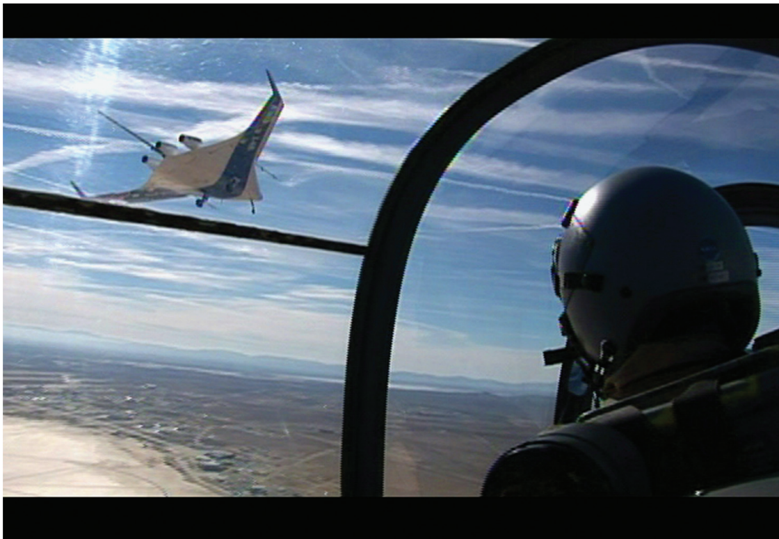
A view from a NASA chase plane during a test flight of the blended wing body X-48B remote-piloted vehicle in April 2008. Image credit: NASA Dryden/Lori Losey
