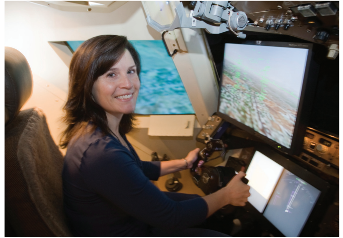
Simulators play a large role in testing new aviation safety technologies, including this test of a synthetic vision system that creates a graphical representation of the environment outside the aircraft. Image Credit: NASA
