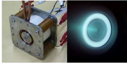
**Figure 4 - Thruster model of TAL at University of Tokyo**
