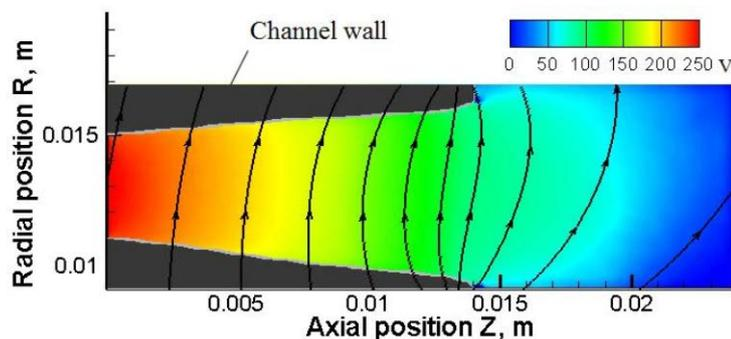
**Figure 5 - Numerical results for electric potential distribution, and channel wall shape at EOL (dark grey area) for a 300 W SPT [16]**
