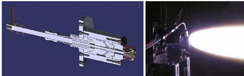
**Figure 3 – 15-kW water-cooled arcjet at JAXA [12]**
