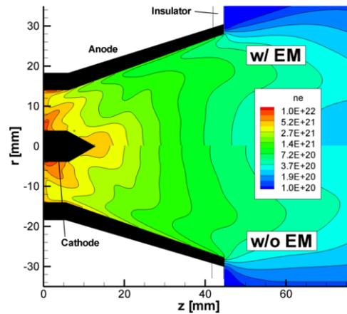
**Figure 2 - Numerical computation result for MPD thrusters by JAXA [10]**
