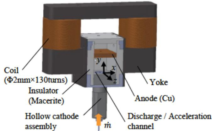
**Figure 1 - Parallel-plate steady-state AF-MPD (1 kW – class) of Nagoya University [7]**
